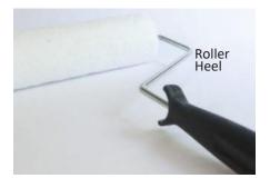
Slightly rotate the handle from left to right applying a little more pressure toward the heel. This will ensure a nice even spread of ReMARKable™ and eliminate "roller lines" in your wall.
